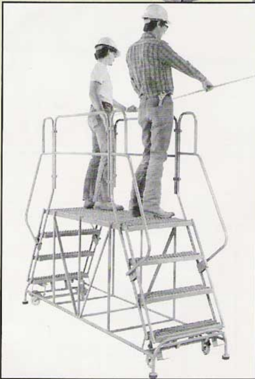
STEPPING DOWN LOWERS TRIP BAR TO IMMOBILIZE LADDER
